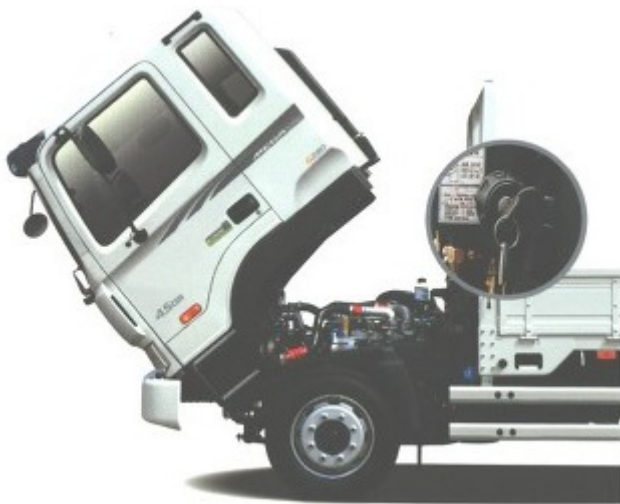
Figure 1: Hyundai mega truck with the cabin in a raised tilted position.
